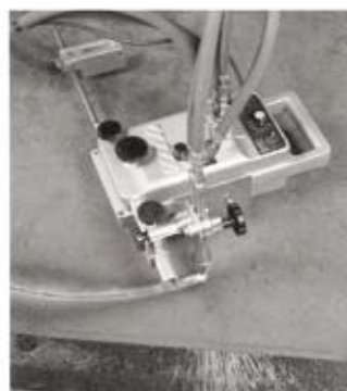
IMP with circle cutting device
