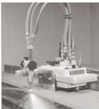
IMP for automatized straight cuts by angled profile guidance
