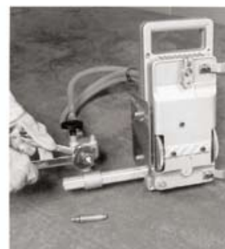
The IMP placed in upright position allows nozzle changing easily
