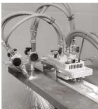
IMP with one-sided torch installation
